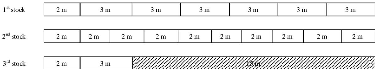
Figure 3. Result of solving the example 1 by the second optimum pattern, total wastage = 15 m
