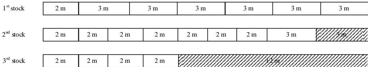
Figure 2. Result of solving the example 1 by the first optimum pattern, total wastage = 15 m
