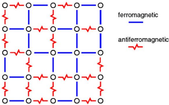
Fig. 1. 2-D spin glass with bond disorder. Spins are placed on the sites of a regular grid. They interact with their neighbors; the interaction is random, either ferromagnetic (straight lines) or antiferromagnetic (jagged lines) [14].
